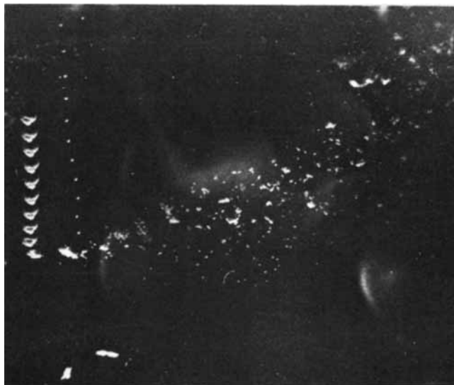
Figure 9. Breakage of kaolin-polyacrylamide floc at Re = 2646 and x_1 \approx 0.005 m.
